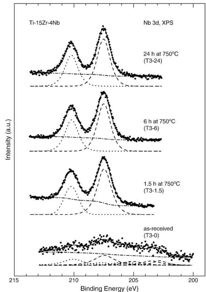
Fig. 4. Nb 3d spectra of Ti-15Zr-4Nb for as-received condition (T3-0) and oxidized at 750 °C for 1.5, 6 and 24 h (T3-1.5, T3-6 and T3-24, respectively). The solid line through the data points represents the results of a least-squares fit.
