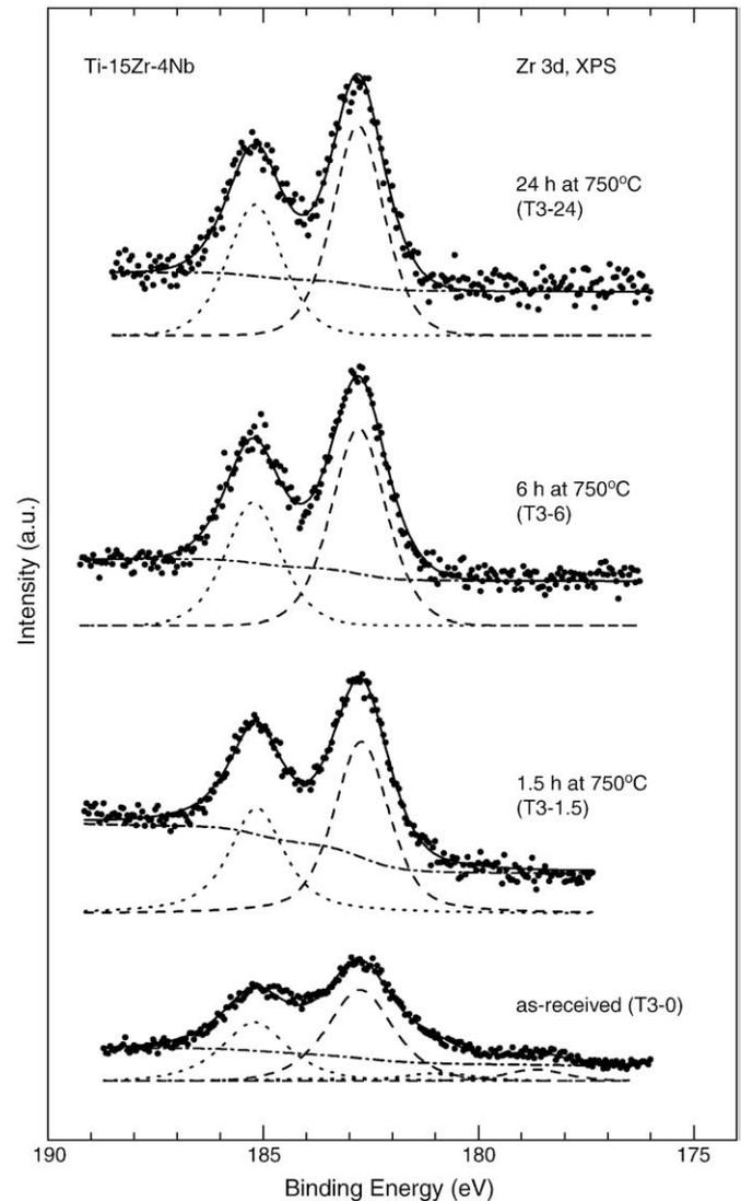
Fig. 2. Zr 3d spectra of Ti-15Zr-4Nb for as-received condition (T3-0) and oxidized at 750 °C for 1.5, 6 and 24 h (T3-1.5, T3-6 and T3-24, respectively). The solid line through the data points represents the results of a least-squares fit.
