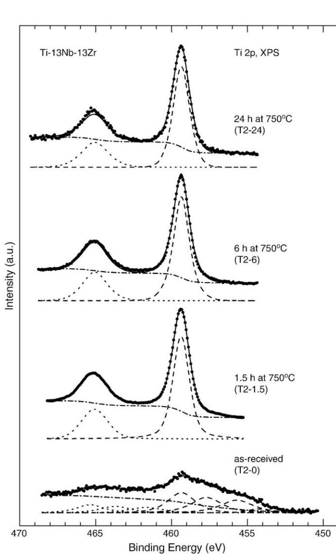
Fig. 1. Ti 2p spectra of Ti-13Nb-13Zr for as-received condition (T2-0) and oxidized at 750 °C for 1.5, 6 and 24 h (T2-1.5, T2-6 and T2-24, respectively). The solid line through the data points represents the results of a least-squares fit.
