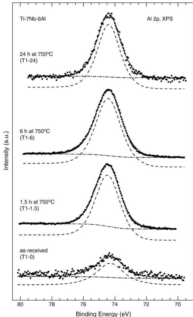
Fig. 3. Al 2p spectra of Ti-7Nb-6Al for as-received condition (T1-0) and oxidized at 750 °C for 1.5, 6 and 24 h (T1-1.5, T1-6 and T1-24, respectively). The solid line through the data points represents the results of a least-squares fit.
